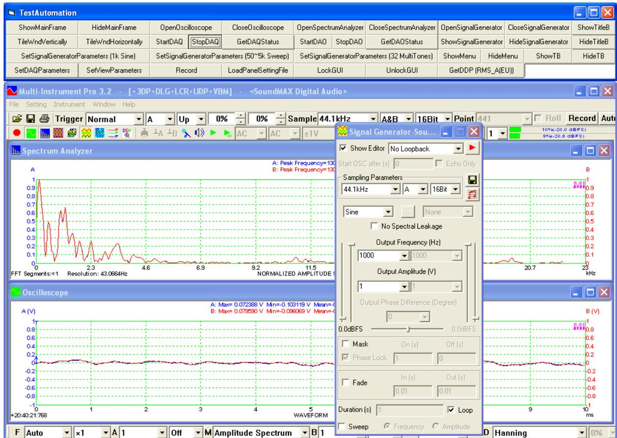
The program TestAutomation demonstrates how to use the Automation interfaces exposed by the Multi-Instrument Automation Server to control the Multi-Instrument program. There are four lines of push buttons on the top of Multi-Instrument program (see screenshot above). The labels on these buttons are self-explanatory. You can use these buttons to control the Multi-Instrument program.
