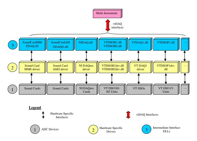
The following diagram shows how Multi-Instrument communicates with different types of DAC hardware via the standard vtDAO interfaces.
