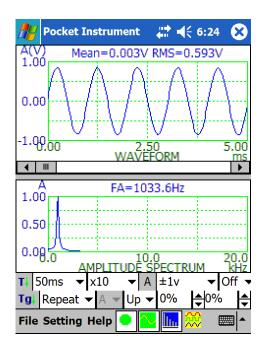
The oscilloscope in the above screenshot shows that the waveform was triggered right at 0V (Trigger Level = 0%) upward (Trigger Edge = Up). The stability of the triggered waveform display was very good. The scan time was set to 50ms. The multiplier of the horizontal axis was set to  $\times 10$  in order to see the individual cycles of the 1kHz sine wave signal. The scan time should be increased if instable triggering occurs.
