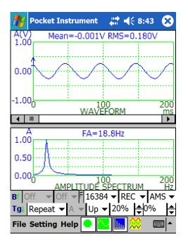
The oscilloscope in the above screenshot shows that the waveform was triggered right at 0.2V (Trigger Level = 20%) upward (Trigger Edge = Up). The stability of the triggered waveform display was very good. The scan time was set to 1s. The multiplier of the horizontal axis was set to  $\times 5$  in order to see the individual cycles of the 20Hz sine wave signal. The scan time should be increased if instable triggering occurs.
