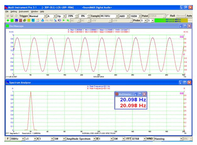
The oscilloscope in the above screenshot shows that the waveform was triggered right at 0.2V (Trigger Level = 20%) upward (Trigger Edge = Up). The stability of the triggered waveform display was excellent and no shaking left and right or up and down was seen.
