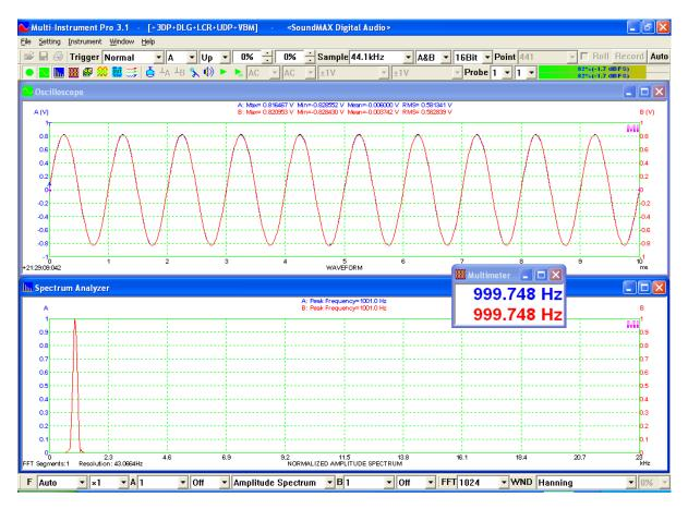
The oscilloscope in the above screenshot shows that the waveform was triggered right at 0V (Trigger Level = 0%) upward (Trigger Edge = Up). The stability of the triggered waveform display was excellent and no shaking left and right or up and down was seen, thanks to the unique algorithm used in the Multi-Instrument software, which is specially designed to overcome the small shaking left and right problem inherent in common software trigger algorithms.
