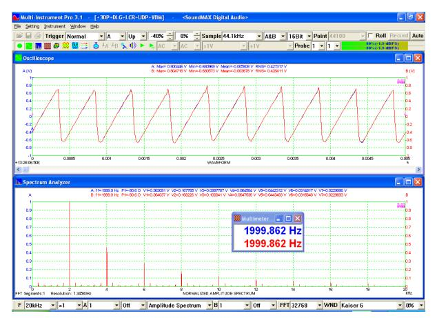
The oscilloscope in the above screenshot shows that the waveform was triggered right at 0.4V (Trigger Level = -40%) upward (Trigger Edge = Up). The sawtooth waveform measured is good in shape.
