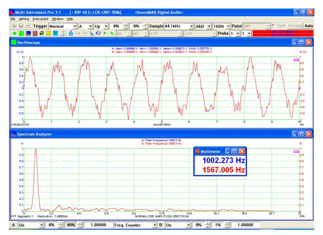
The oscilloscope in the above screenshot shows that the waveform was triggered right at 0V (Trigger Level = 0%) upward (Trigger Edge = Up).
