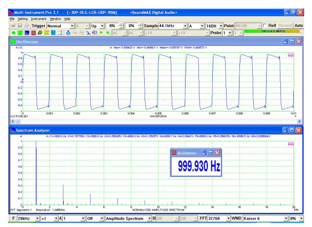
The oscilloscope in the above screenshot shows that the waveform was triggered right at 0V (Trigger Level = 0%) upward (Trigger Edge = Up). The square waveform measured is reasonably good in shape despite that the top and bottom of the waveform is not so flat as the ideal one, which can be attributed to the limited bandwith and phase distortion of both the output channel of the Pocket PC and the input channel of the laptop.
