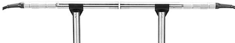
测量超低声压级所用的面对面紧靠的话筒对
